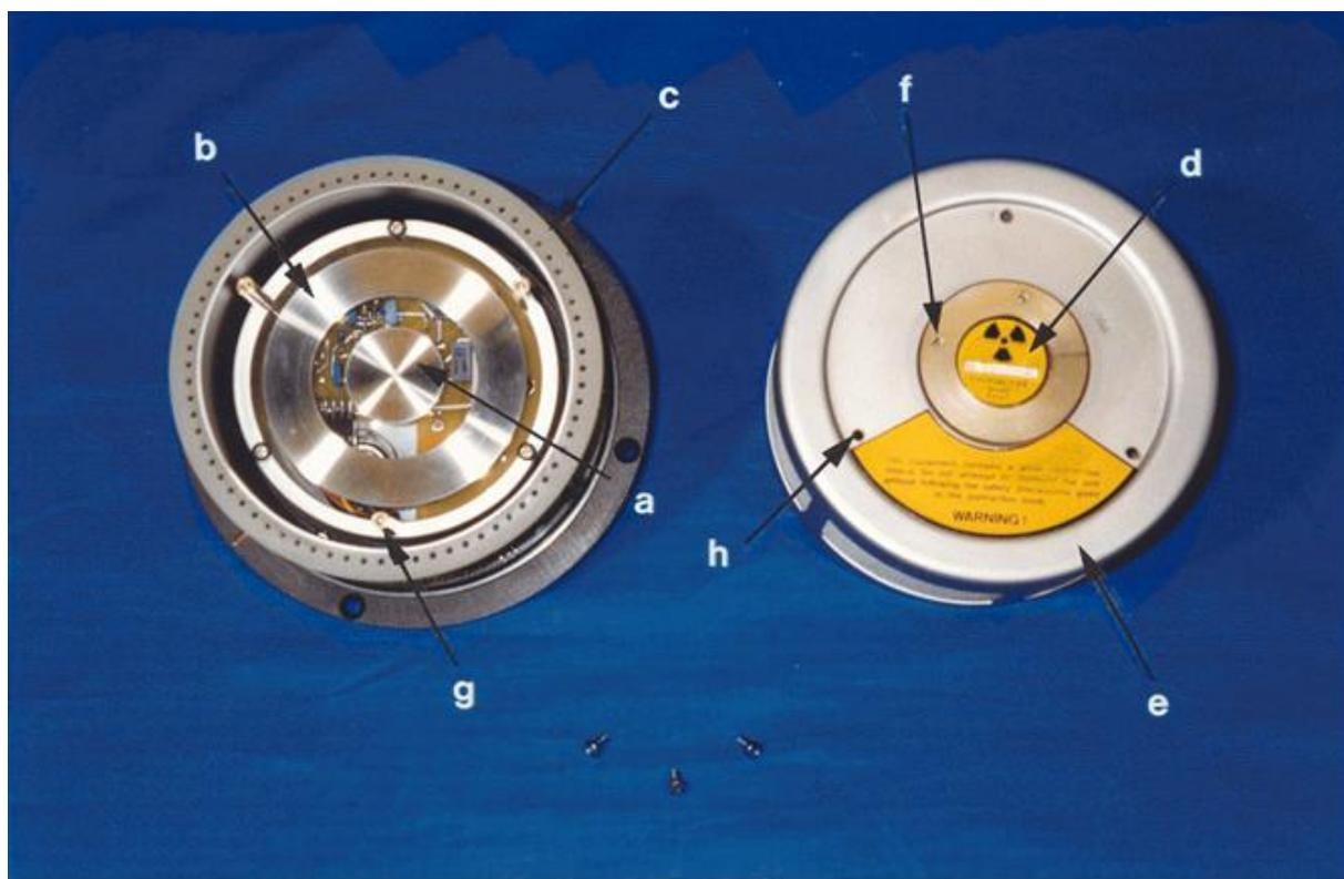
Fig. A.1.2 Measuring Ionization Chamber (MIC) EC-912-10 with chamber housing removed
