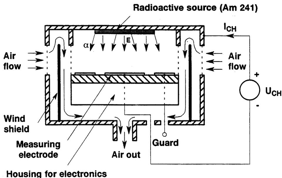
Fig. 4.2.1 Principle of ionization chamber design in the MIC
