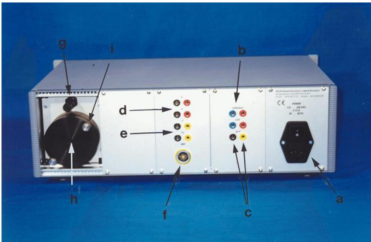
Fig. A.1.4 Rear of control cabinet EC-910-10 with flow control unit EC-912-40
