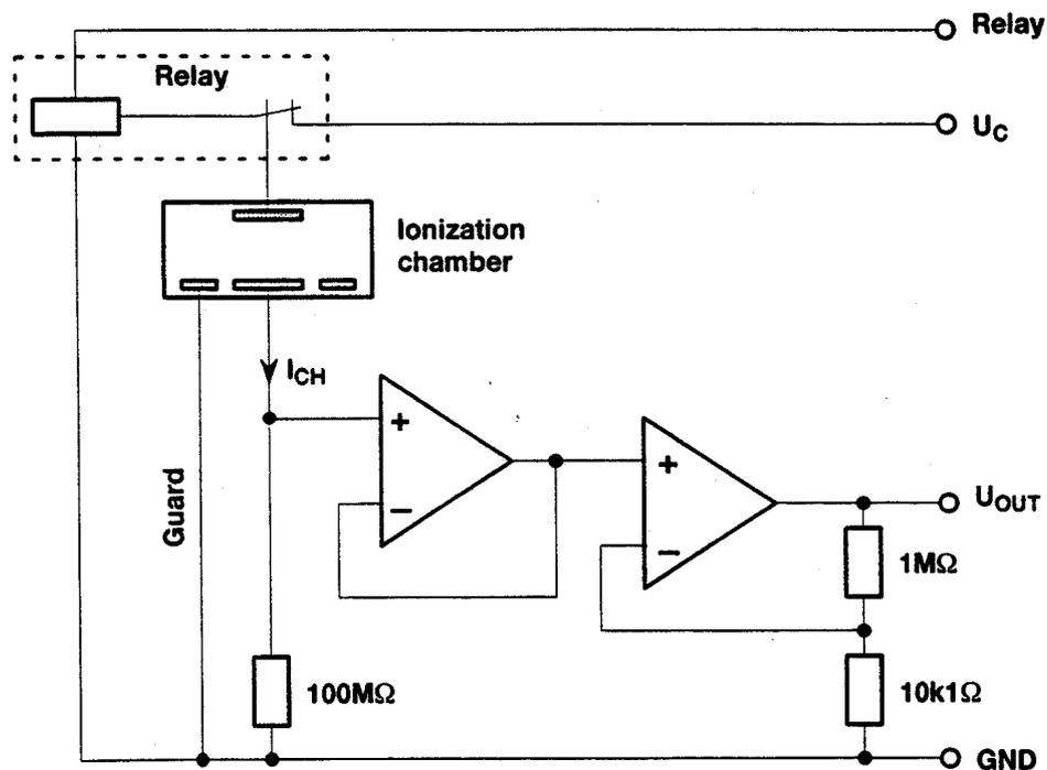
Fig. 4.2.2 Principle of MIC impedance transforming circuit
