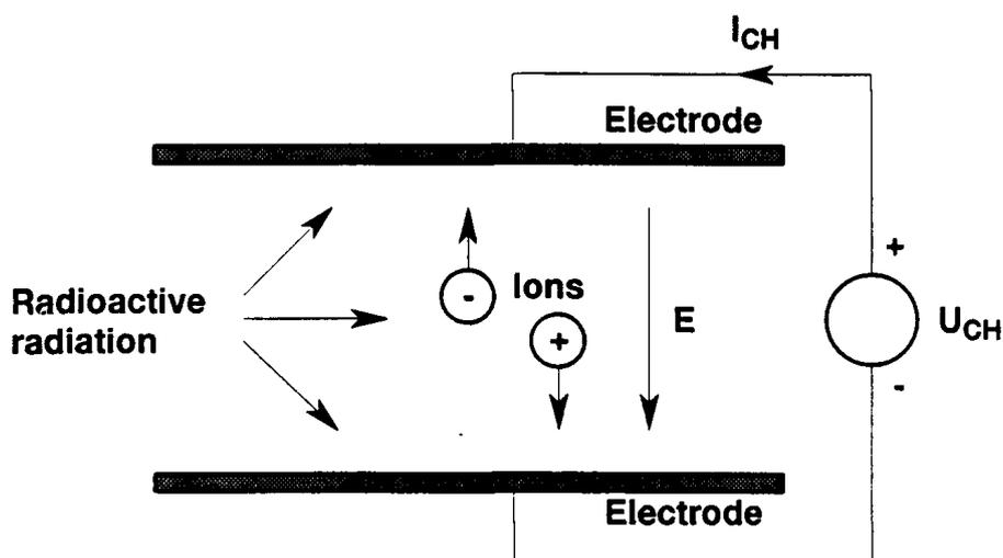
Fig. 4.1 Working principle for ionization chamber
